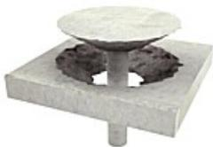
Adding further reinforcement in the form of loose shear links around column heads has been used as a measure to resist punching shear but these links are time consuming and labour-intensive to install and design.
