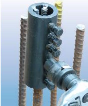
Insert the Unitec coupler over the end of the first bar until contact with the centre pin. Strongly hand tighten the screws from centre to outside with a wrench to preposition the coupler progressively in order to maintain its alignment with the bar.
