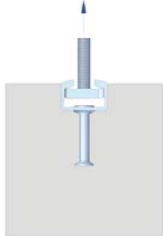
Breakout of channel lips under tensile loading
