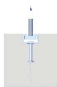
Splitting of concrete under tensile loading
