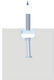
Breakout of channel stud under tensile loading
