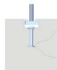
Blow out of concrete under tensile & shear loading
