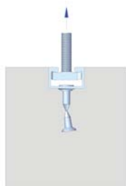
Breakout of stud under tensile loading
