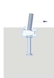
Breakout of channel lips under shear loading
