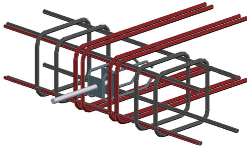
Figure 5.2: Arrangement of the cross-ties of the concrete edge reinforcement and edge beam reinforcement. Three-dimensional view.
