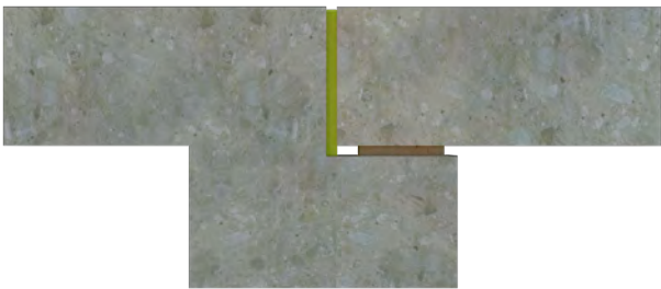
• Conventional corbel support solution
