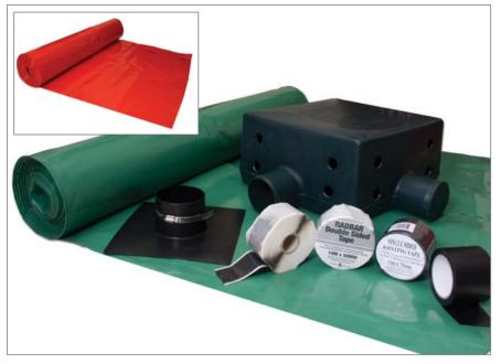
**THE RADBAR RADON SYSTEM** consists of a membrane extending the whole of the floor and walls. The system should incorporate an under floor ventilated sump or sumps, which can be subsequently converted to an active system by use of suitable ventilation fans. Radbar radon resisting membrane when installed in accordance with the BRE and NHBC recommendations, will also act as a damp proof membrane to protect the building against the ingress of moisture from the ground.
