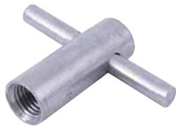
RFA-Tech Fixing Inserts with Cross Pin (Heavy Duty) provide a cost effective threaded fixing system in cast concrete with a strength of 30N/mm<sup>2</sup> and above, where either the unit or speed of installation required does not permit the use of a high yield reinforcement tail bar. They are effective for a single point fixing where no tolerance is required for attachment.
