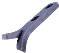
The most versatile of the anchors, the Spread Anchors are suitable for lifting most types of beams, wall panels and slabs. The second hole provides the option to use extra reinforcement where required. These are available in safe working loads from 0.7t to 26.0t.
