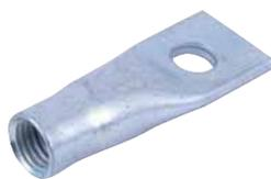
RFA-Tech Fixing Inserts with Cross Hole provide a threaded fixing system in cast concrete with a strength of 30N/mm<sup>2</sup> and above. They are effective for a single point fixing where no tolerance for attaching is required.
