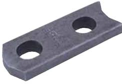
Two Hole Anchors are suitable for use where load distribution is not possible through the foot of a spread anchor and is done so by use of a reinforcement tail bar. They are particularly useful in thin wall panels and trusses, or where concrete strength is low. These are available in safe working loads from 0.7t to 22.0t.
