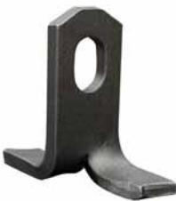
Flat Foot Anchors are used for thin slabs and additional reinforcement is essential. They are available in safe working loads from 1.4t to 22.0t.
