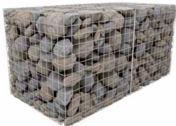
Gabions are wire mesh baskets manufactured from 3.0mm Galfan Wire, and are filled on site with typically stone or rock to form larger building modules. Galfan wires are best used where the additional PVC coating is not a requirement, such as freshwater river applications and low height retaining walls on dry land, where aesthetics are not paramount.
