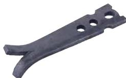
Erection Anchors are specifically designed for pitching and turning concrete units. They have specially designed ribs on the head of the anchor which prevent concrete from spalling when turning units. These are available in safe working loads from 1.4t to 22.0t.
