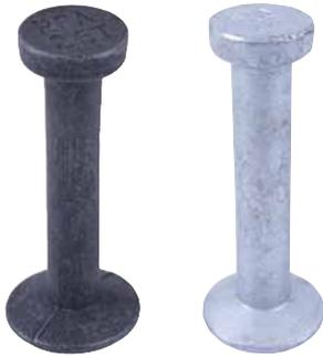
The Capstan Anchors are a safe, simple and effective system for lifting most types of precast concrete units. The anchors are hot drop forged from high grade steel and, provided the anchor is specified and installed correctly, ensures safe and secure lifting, turning and transportation of units.
